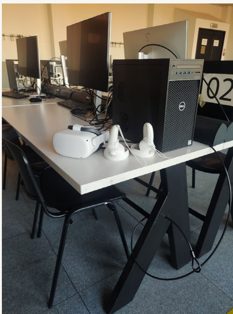
▲ Fig. 3.1.2: Workstation, composed of the desk computer, the headset and the controllers.
